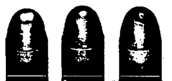
No. 24. Exposed Steel (clad jacket)
