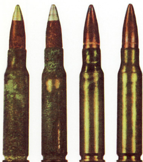
No. 2. Corroded or Stained
