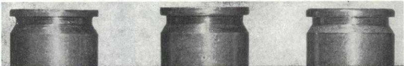
[ — — — — — Major — — — — — ] [ — Permissible — ] No. 13b. No Chamfer on Head (rim) (Twice normal size)
