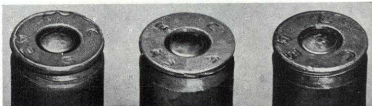
No. 12b. No Chamfer on Head (rim) (Twice normal size, inclined view)
