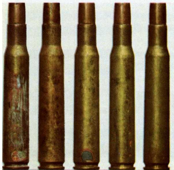
No. 2. Corroded or Stained
