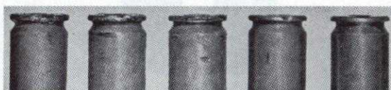
No. 16a. Defective Head
