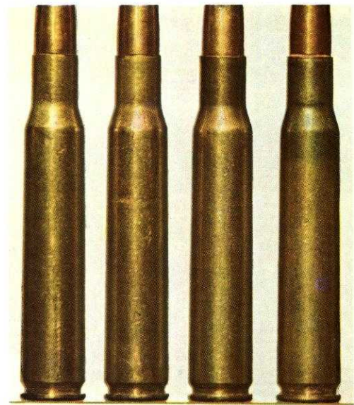
No. 21. No Visible Evidence of Mouth Anneal
