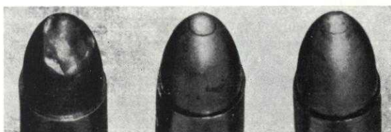
No. 24c. Upset (crooked) Point (Twice normal size)
