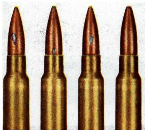
No. 29. Exposed Steel (clad jacket)
