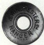
Deformed Head
