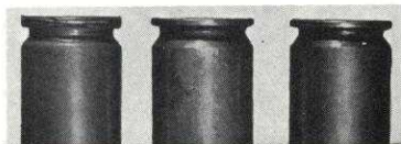
No. 12a. No Chamfer on Head (rim)
