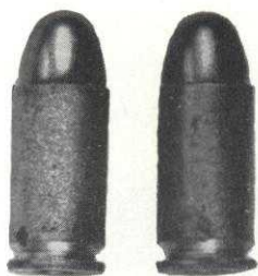
Defective Zinc Plating
