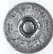
g. Battery Cup Defects
