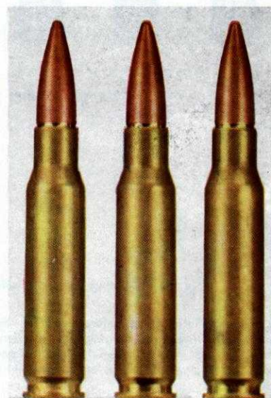
No. 21. No Visible Evidence of Mouth Anneal
