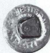
g. Battery Cup Defects
