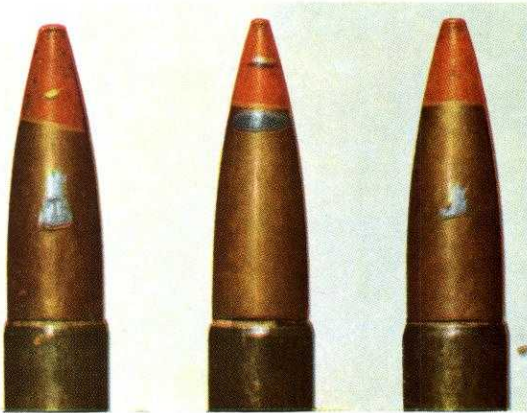
[ — — — — — Minor — — — — — ] No. 29. Exposed Steel (clad jacket)
