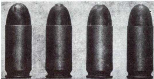
No. 23a. Upset (crooked) Point (Normal size)
