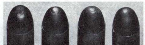
No. 23b. Upset (crooked) Point (Normal size, inclined view)
