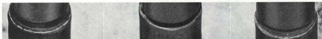
No. 11c. Case Mouth not Crimped in Cannellure (Twice normal size, inclined view)
