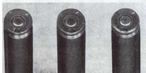
No. 13b. No Chamfer on Head (rim)
