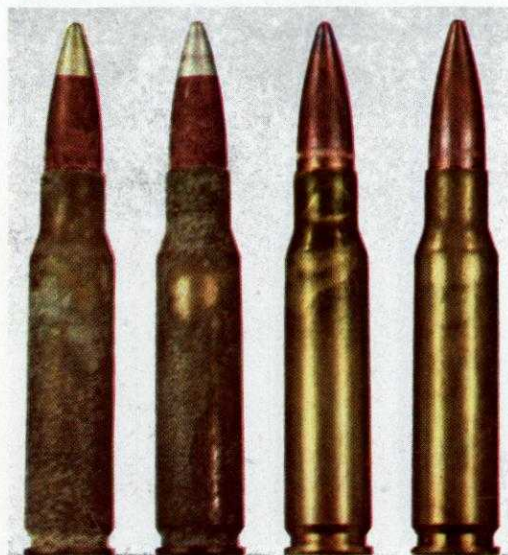
No. 2. Corroded or Stained
