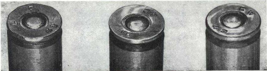
[ — — — — — Major — — — — — ] [ — Permissible — ] No. 13d. No Chamfer on Head (rim) (Twice normal size, Inclined view)
