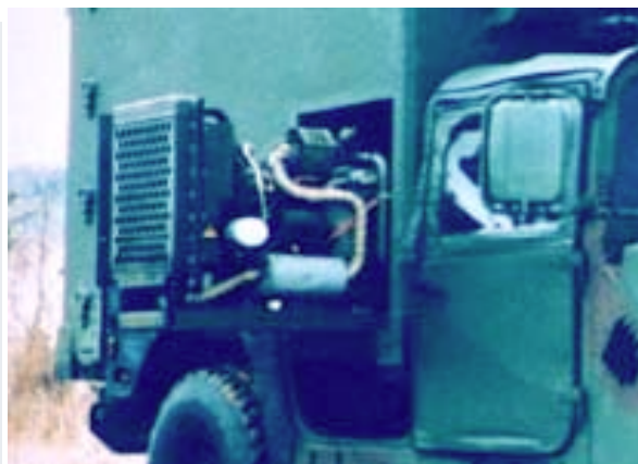
10 kW APU ready to slide into shelter.
