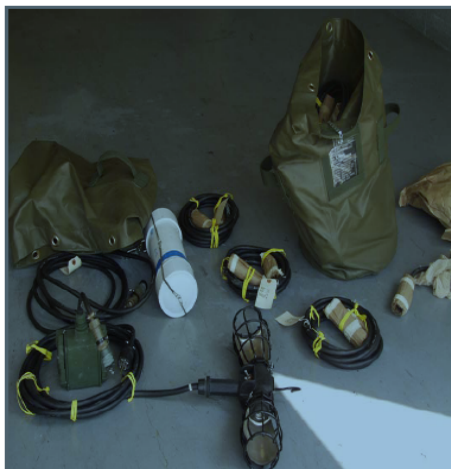
FIGURE C- 56 DISE, 40 Amp per Phase Distribution System - 3 Phase
