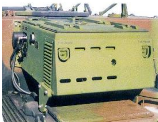
MEP-952A on M557 (Power connector side)
