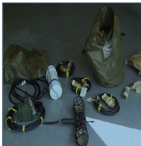
FIGURE C- 56 DISE, 40 Amp per Phase Distribution System - 3 Phase
