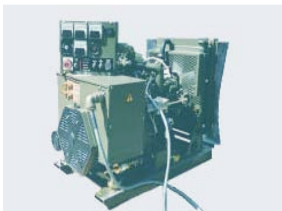
10 kW APU and control panel removed from shelter. --
