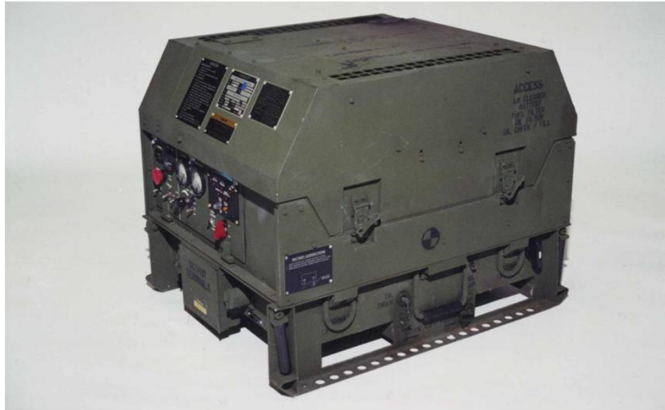
MEP-831A (60 Hz) has convenience outlet and fault protection Radii: Access door = 25.4", Output Terminal door = 10.0", Control Panel door = 8.5".
