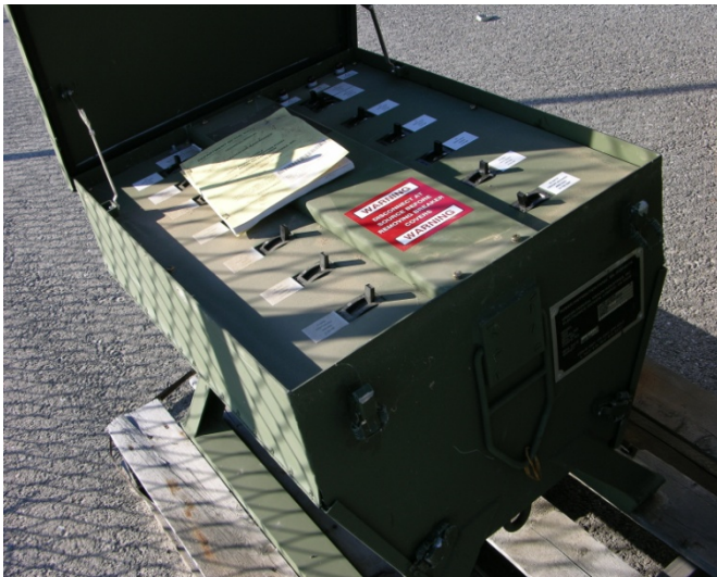
FIGURE B- 33 120kW Power Distribution Panel
