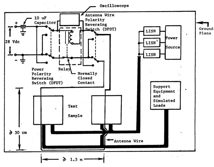
NOTES: 1/ No suppression components (shielding, diodes, etc) shall be attached to the relay or its wiring.
