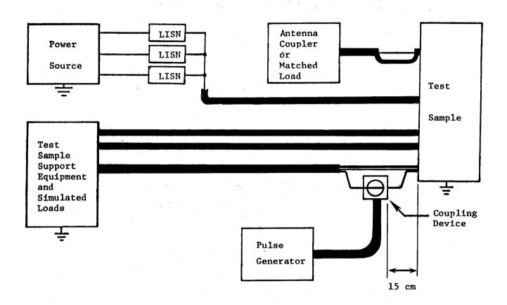
FIGURE CS13-2. Test setup for CS13.
