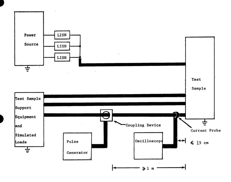
FIGURE CS12. Test setup for CS12.
