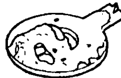
FIGURE 5-24. Plated-thru holes - clinched leads and wires.
