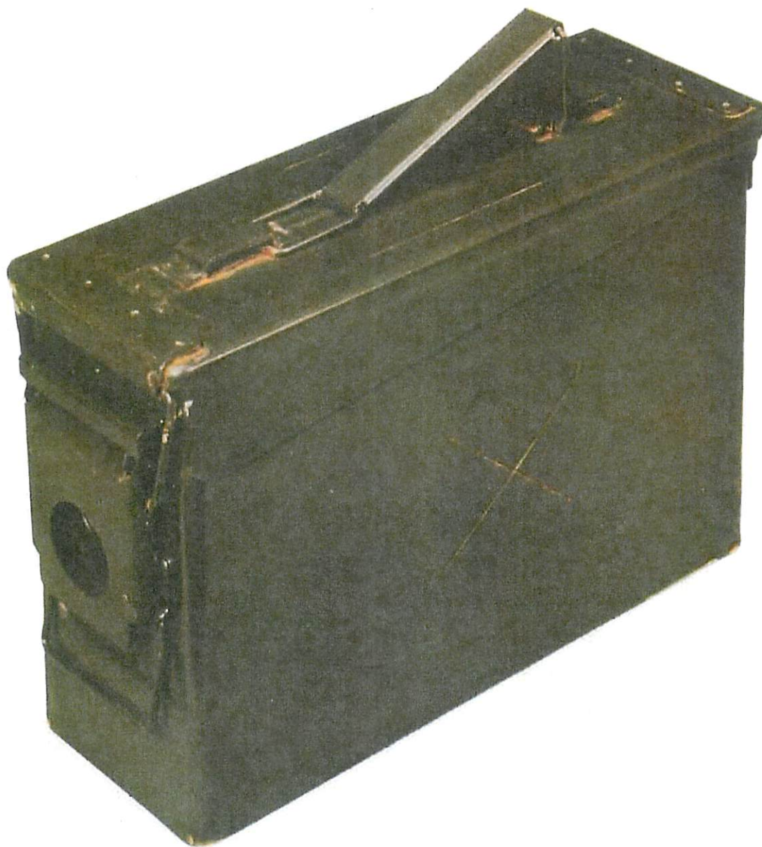
"WORST" PERMISSIBLE DEGREE OF RUST AFTER CORROSION RESISTANCE TEST
