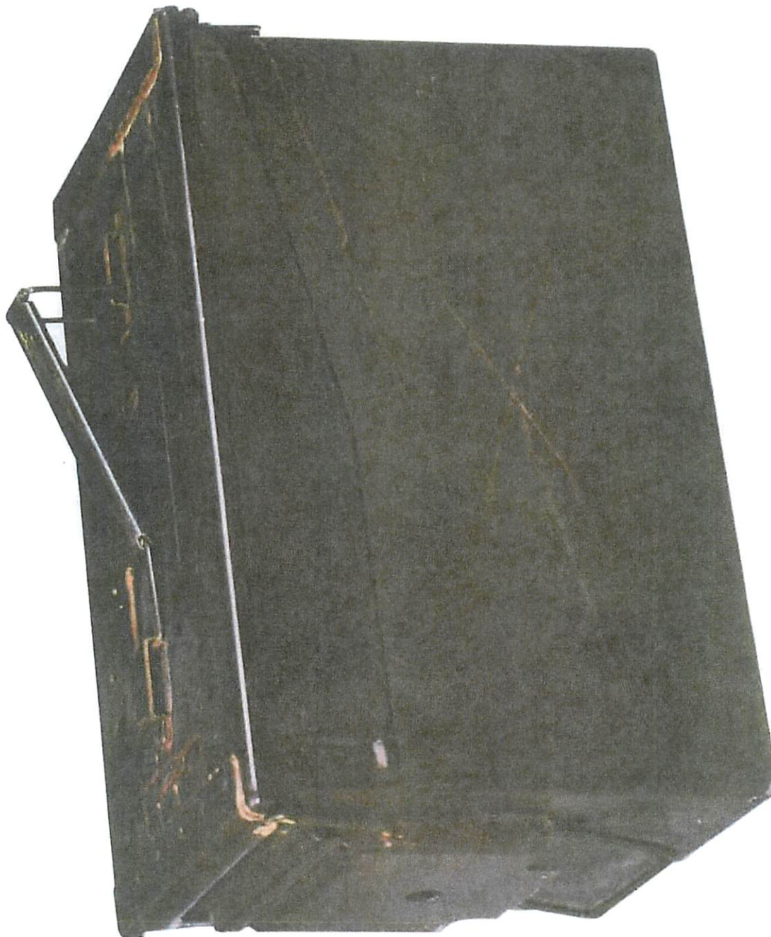
"WORST" PERMISSIBLE DEGREE OF RUST AFTER CORROSION RESISTANCE TEST
