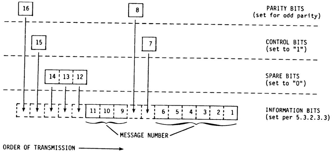
FIGURE 3. Message number field in digital common channel signaling and supervisory messages.
