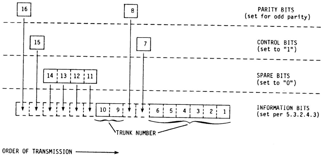
FIGURE 4. Trunk number field in digital common channel signaling and supervisory messages.
