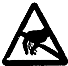
FIGURE 43. ESD sensitive devices attention symbol and label for unit packs.
