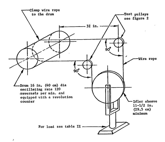
FIGURE 1. Diagram of Endurance Testing
