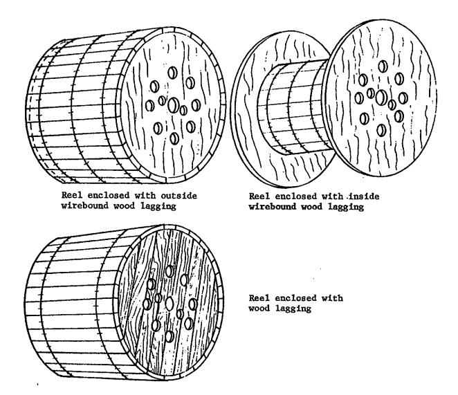
FIGURE 3. Typical Reel of Wire Rope Enclosed with Wood Lagging or Wirebound Wood Lagging
