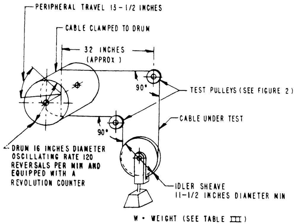
FIGURE 1. Cable Endurance Testing Machine (Diagrammatic)
