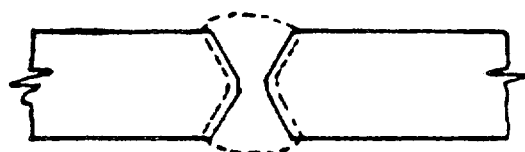
C. Double-V butt joint, welded both sides (type B-31).
