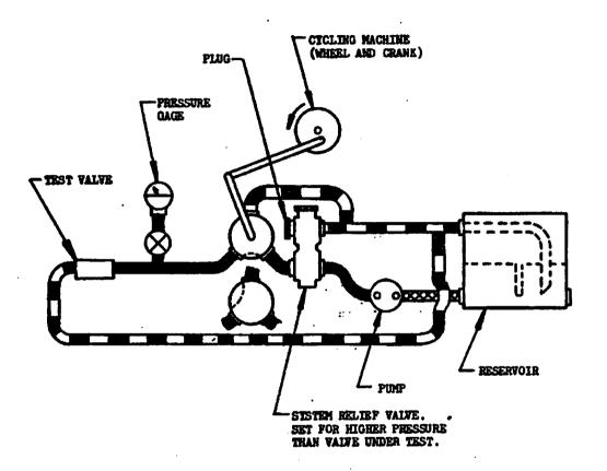
FIGURE 3. Typical relief valve Endurance test installation
