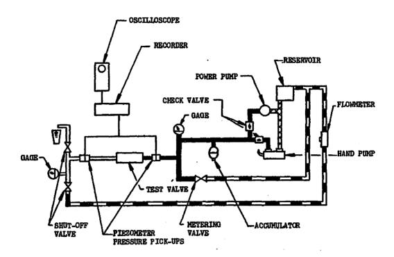
GAGES SHALL BE PLACED AS CLOSE TO VALVE PORTS AS PRACTICABLE.
