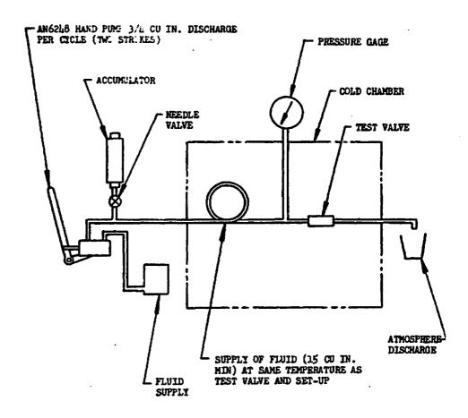
FIGURE 2. Typical schematic diagram for Low temperature performance test
