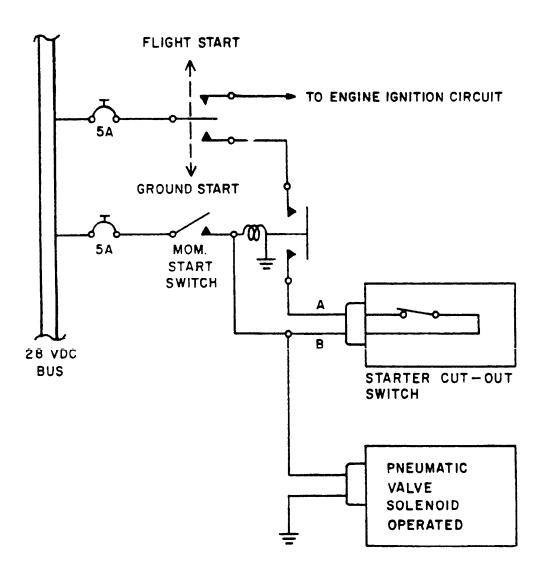
FIGURE 1. Wiring diagram for typical aircraft starting system
