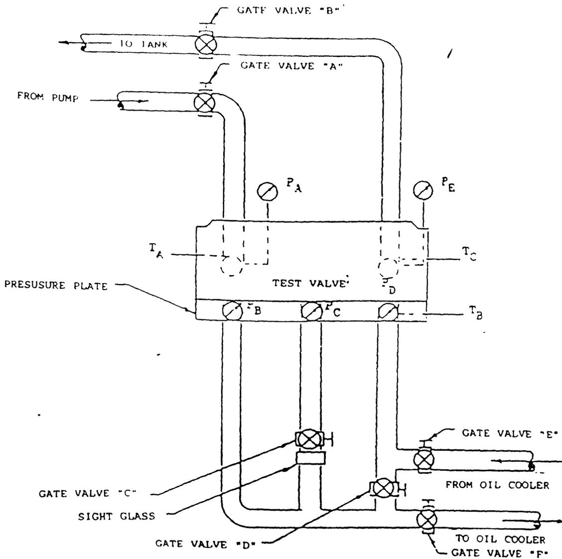
**FIGURE 1. Temperature regulation test apparatus**
