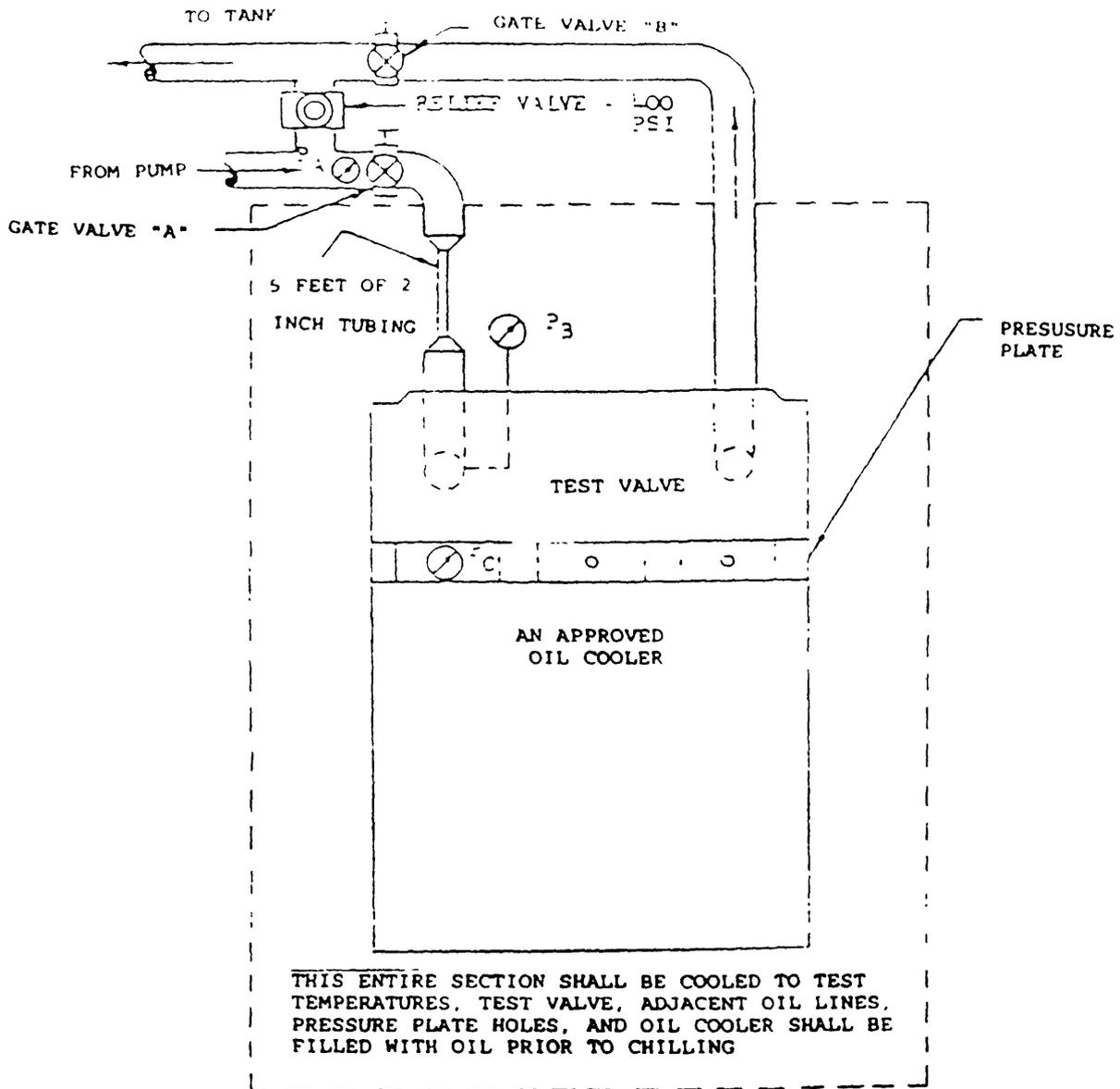
**FIGURE 3. High viscosity surge test apparatus**
