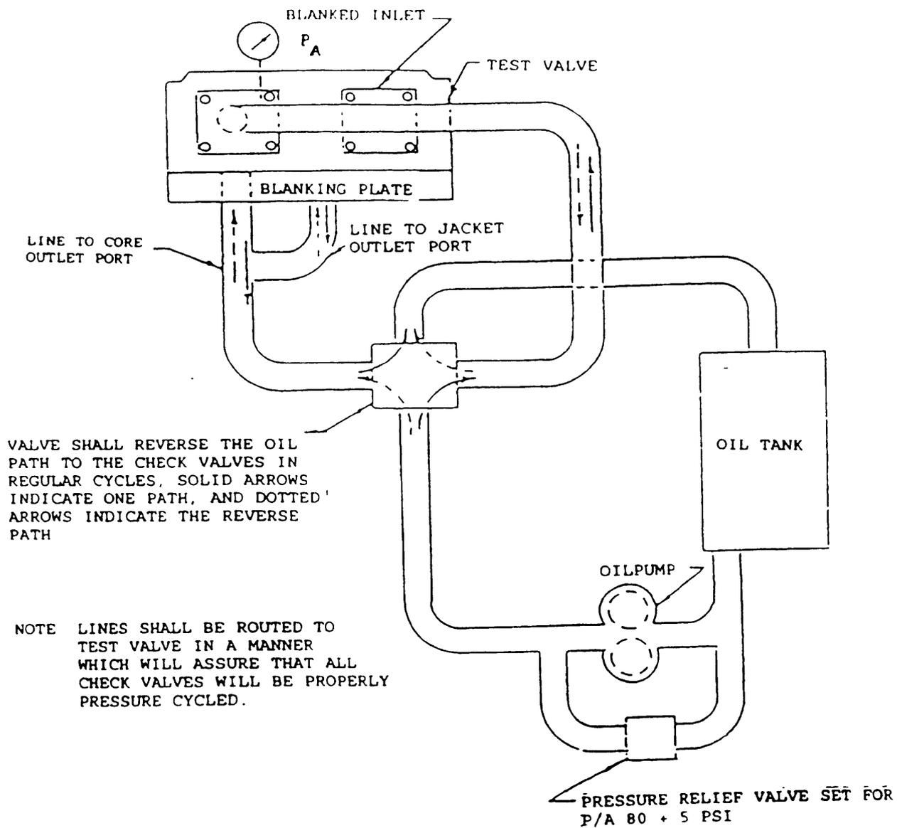
FIGURE 4. Endurance check of test valves
