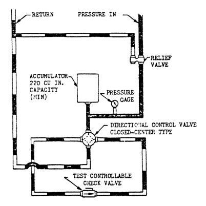
ALL TUBE OD'S SHALL BE AT LEAST ONE SIZE LARGER THAN THE CHECK VALVE TUBE SIZE. TUBE LENGTHS SHALL BE A MINIMUM. HOSE SHALL NOT BE USED.
