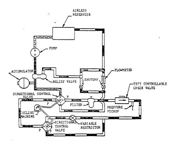
FIGURE 2. Typical setup for Endurance cycling test, automatic checking operation
