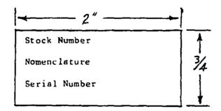
The letters and numbers for the stock number and nomenclature shall be 1/8 inch (3.18mm) high. The numbers and letters of the serial number shall be 3/16 inch (4.76mm) high. There shall be 1/16 inch (1.6mm) space above the stock number and between the stock number and the nomenclature. There shall be a 3/32 inch (2.4mm) space between the nomenclature and the serial number and a 3/32 inch (2.4mm) margin below the serial number.
