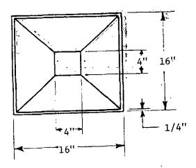
LOADING PLATFORM IS A HOLLOW FRUSTRUM OF A PYRAMID CLOSED AT SMALL BASE, FORMED BY WELDING
