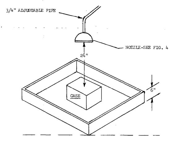
TANK SHOULD BE LARGE ENOUGH TO HOLD CASE WITH A MINIMUM CLEARANCE OF 2" ON EACH SIDE
