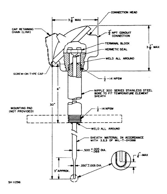
FIGURE 1. Stack gas type resistive temperature assembly.
