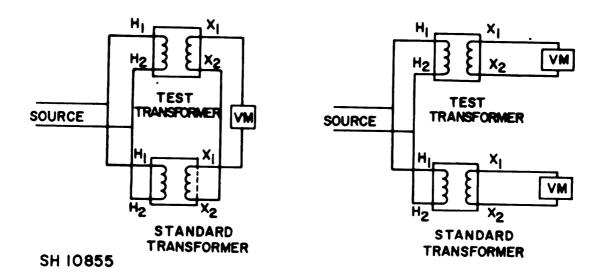
Voltmeter arranged to read the difference between the two secondary voltages.
