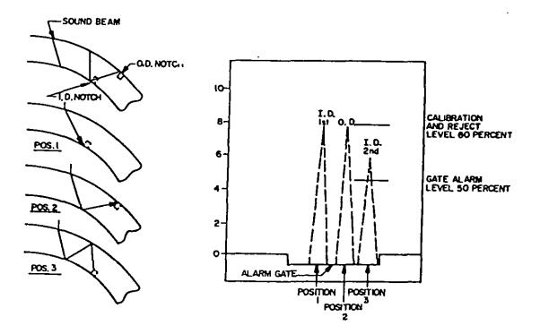
FIGURE 3. <u>Calibration and flaw alarm/rejection/acceptance</u> <u>signal amplitude levels</u>.
