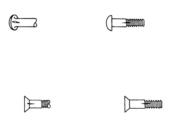
FIGURE 1. LONGITUDINAL DISCONTINUITIES EXTENDING THROUGH FILLETS OR THREADS.
