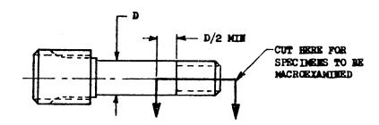
FIGURE 6. Metallurgical Specimen
