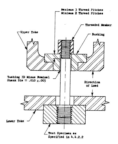
FIGURE 5. Resistance to Pullout Fixtures (4.6.2)
