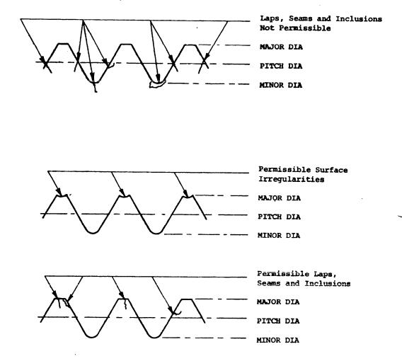
FIGURE 2. Laps, Seams and Surface Irregularities in Thread
