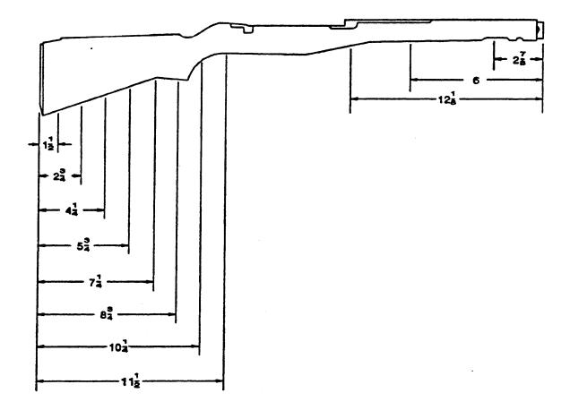
FIGURE 1. <u>Sectioning diagram for obtaining test specimen</u> for adhesive and foam test.
