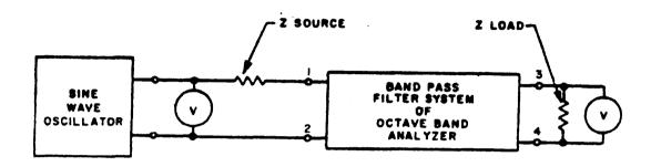
Figure 3. Insertion Loss Test Arrangement for Filter System of Octave Band Analyzer
