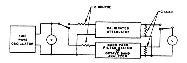
Figure 4. Alternate Insertion Loss Test Arrangement for Filter System of Octave Band Analyzer
