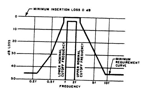
Figure 2. Insertion Loss (Minimum Requirement Curve)
