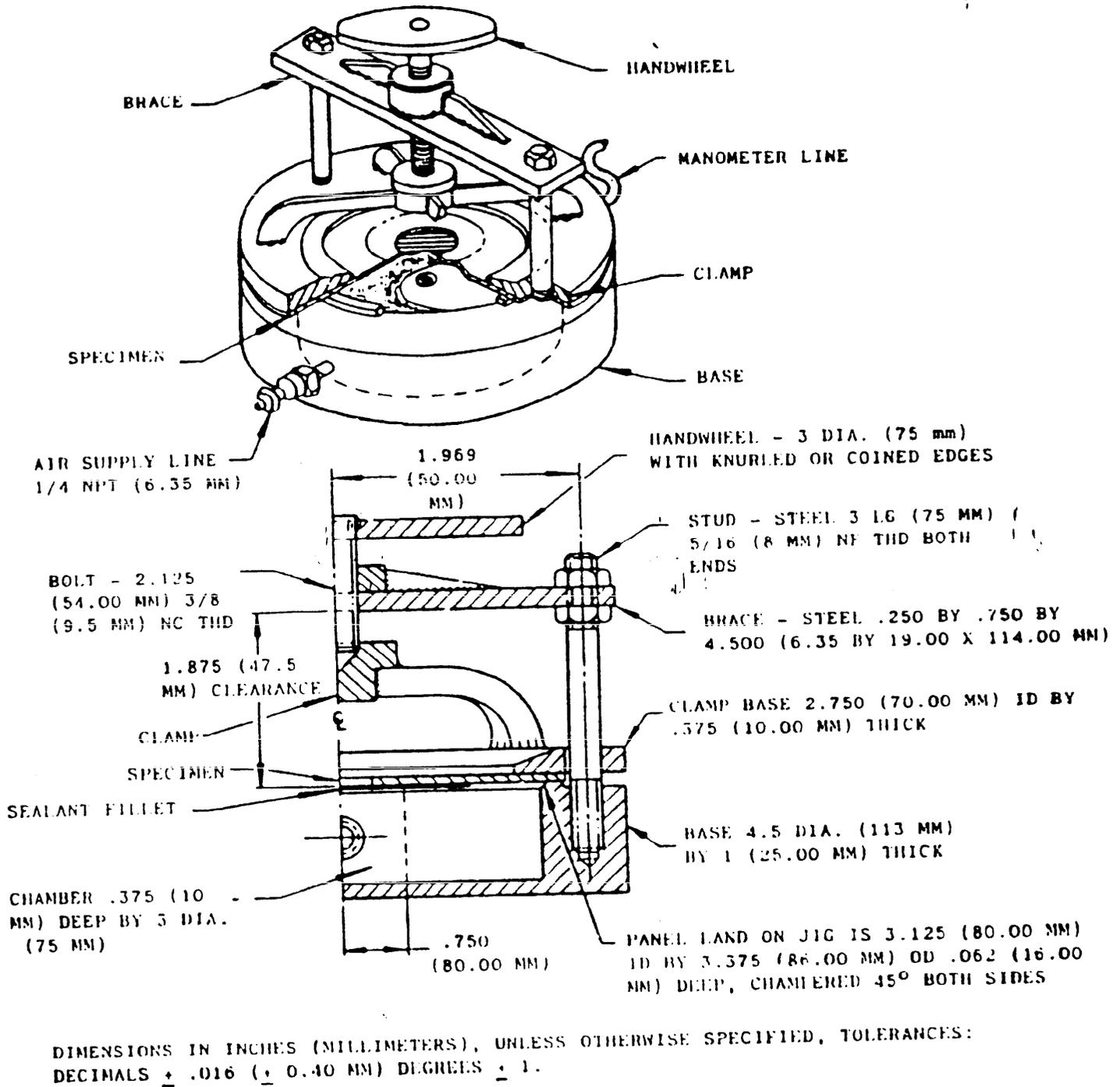
Figure 5. Thermal Rupture Apparatus.
