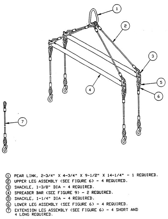
FIGURE 2. Size 17 - 17 ton sling assembly.
