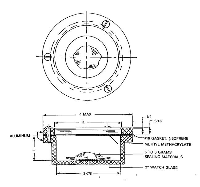
FIGURE 1. Assembly for test on effect of volatile components.
