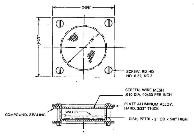
NOTE: TOP & BOTTOM PLATES ARE IDENTICAL, EXCEPT THAT SCREW HOLES ARE TAPPED INTO BOTTOM PLATE
