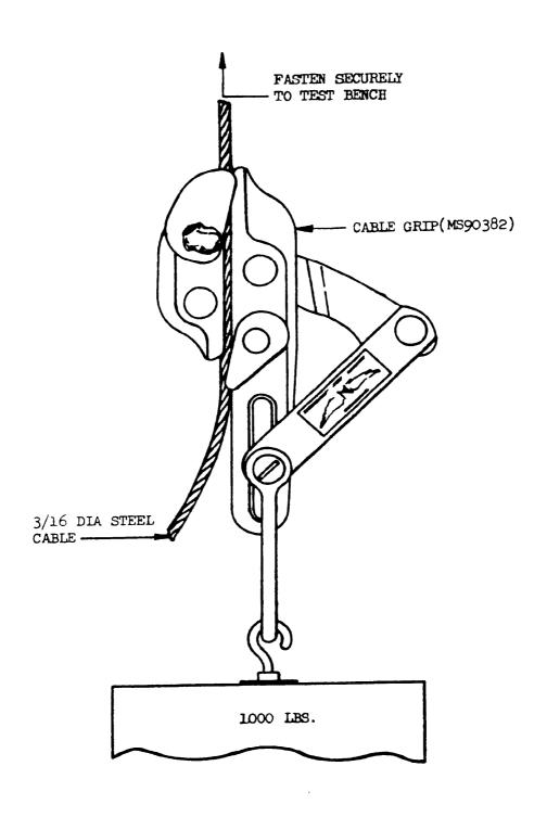
Figure 1. CABLE GRIP PROOF LOAD TEST
