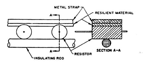
FIGURE 1. Resistor-contacting assembly for insulation-resistance measurements.
