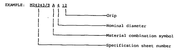
M24243/9A412 Indicates - Rivet, blind, nonstructural, retained mandrel, open-end, 120° countersunk head, 5052 (UNS A95052) aluminum alloy body, 1016-1025 (UNS G10160-G10250) steel mandrel; nominal body diameter size, .125; grip range, .093-.250.
