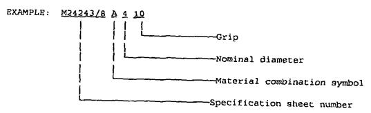
M24243/8A410 Indicates - Rivet, blind, nonstructural, retained mandrel, open-end, snap head, 5052 (UNS A95052) aluminum alloy body, 1016-1025 (UNS G10160-G10250) steel mandrel; nominal body diameter size, .125; grip range, .031-.187.
