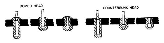
FIGURE 1. ILLUSTRATION OF RIVET STYLES BEFORE AND AFTER SETTING
