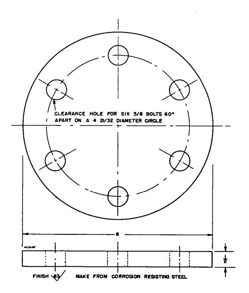
FIGURE 1. Piece 1 of device used to test sealability of gasket material for water stills.
