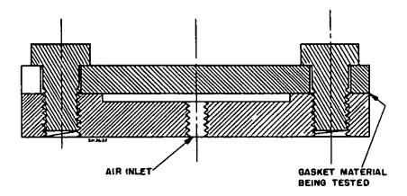
FIGURE 3. Cross-section view of assembled device used to test sealability of gasket material for water stills.
