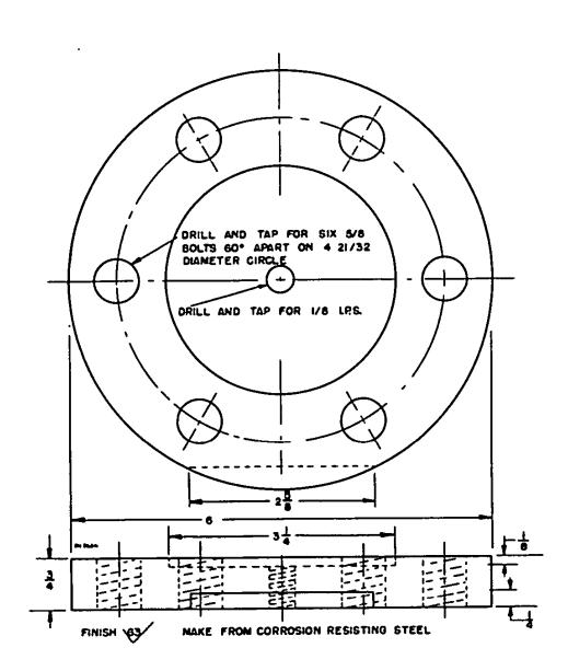
FIGURE 2. Piece 2 of device used to test sealability of gasket material for water stills.
