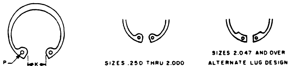
Figure 1. Type I, Class 1 retaining rings.
