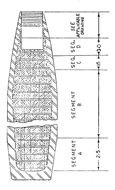
FIGURE I. Projectile, 155MM, M107, HE Charge segments.
