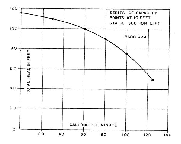
FIGURE I. Pump capacities,
