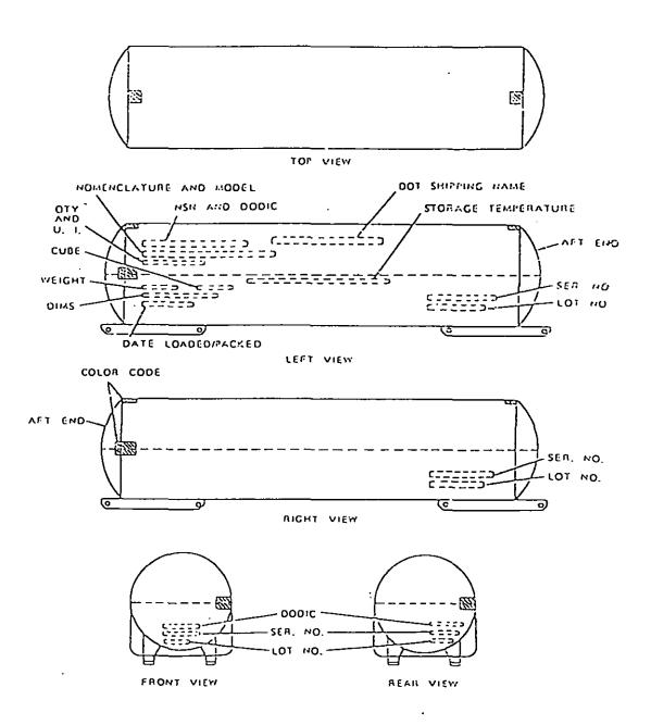
FIGURE 1. Marking of cylindrical containers.
