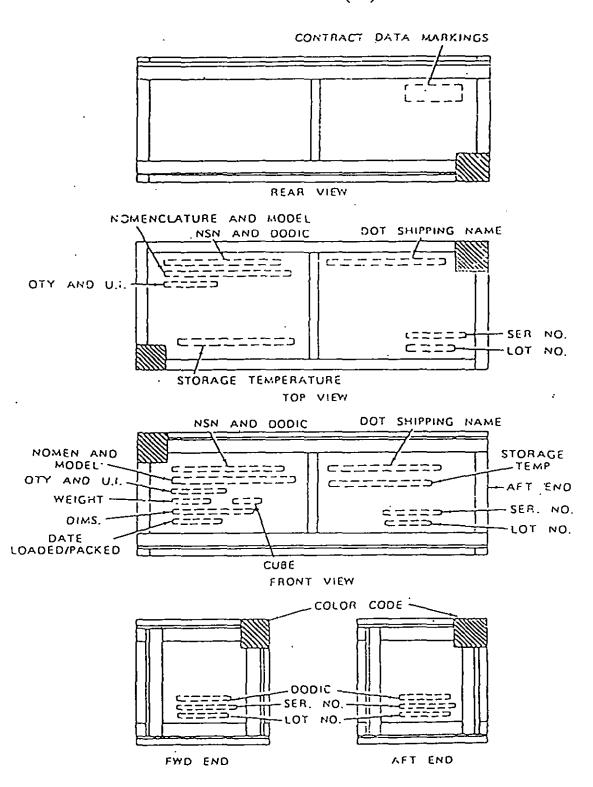
FIGURE 2. Marking of rectangular containers.
