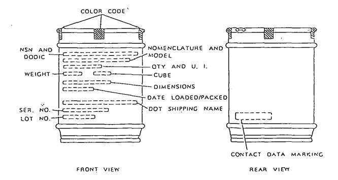
FIGURE 3. Marking of drums.
