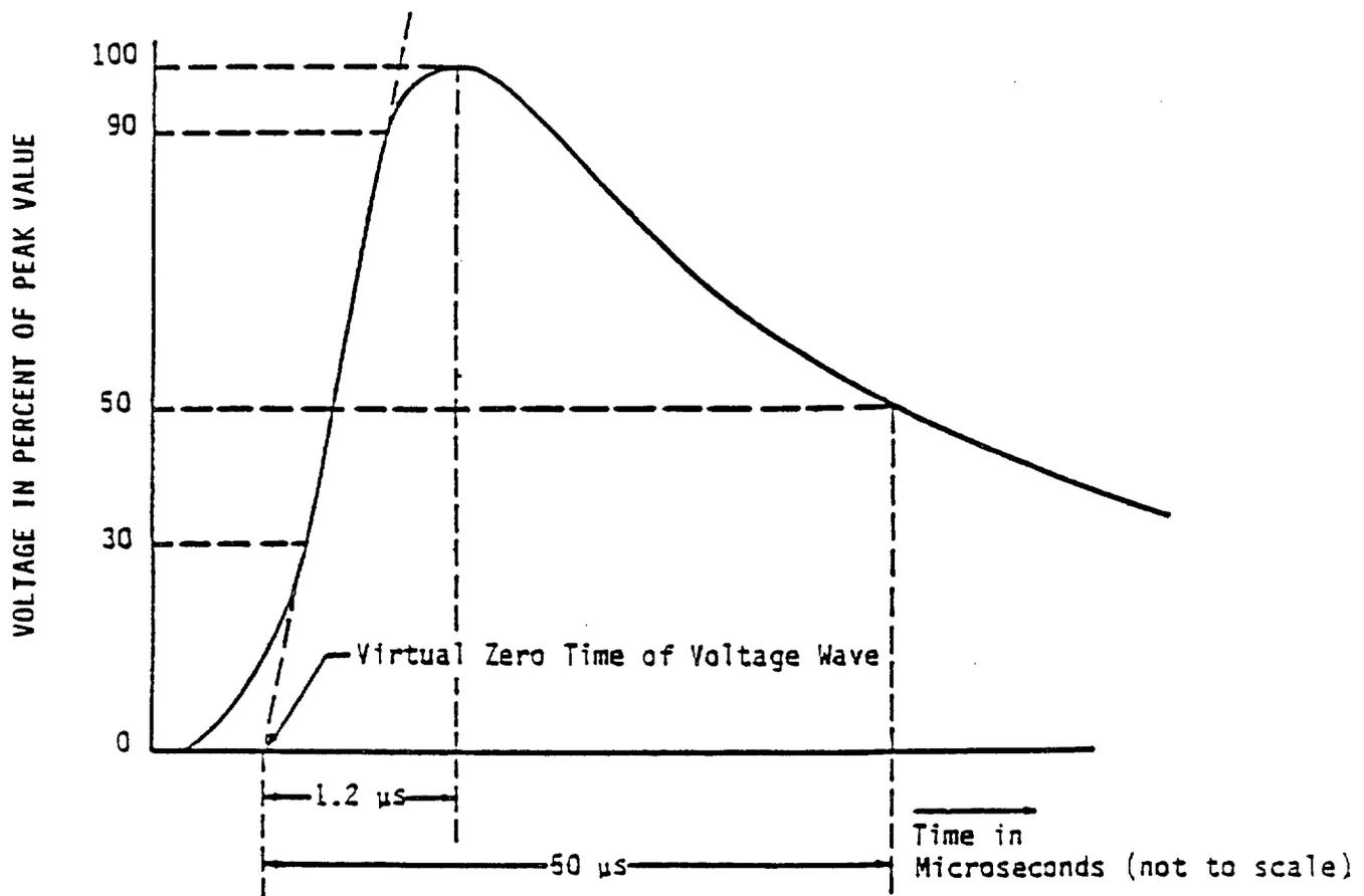
FIGURE 1. Spike voltage (short time transient) wave shape.
