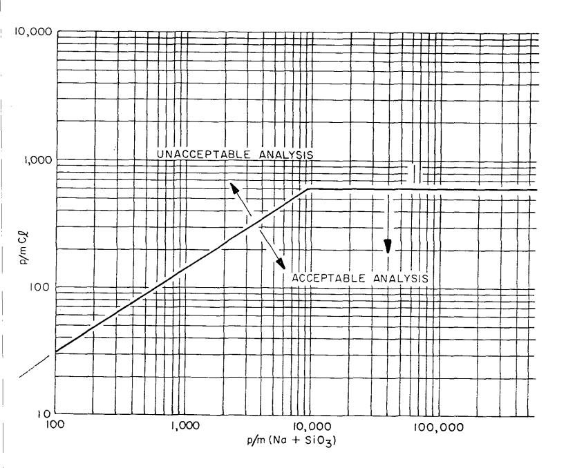
FIGURE 1. Acceptability of insulation on the basis of the plot points of the chloride, sodium, and silicate ions.
