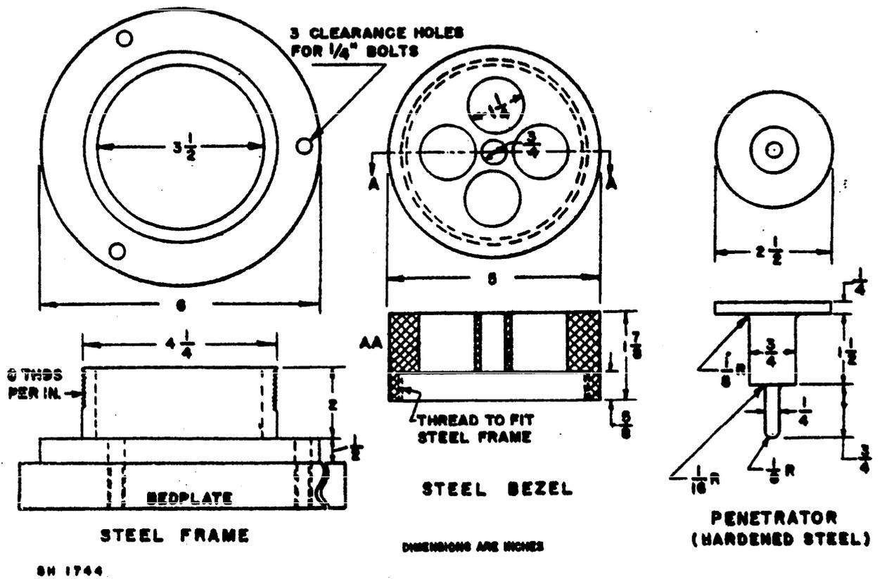
Figure 1 - Penetration impact strength test apparatus.
