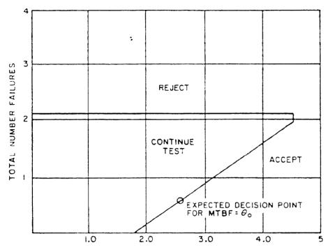
TOTAL TEST TIME (IN MULTIPLES OF LOWER TEST MTBF  $\theta_1$ )
