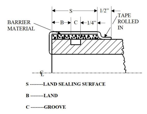
FIGURE 2. Land sealing surface for grooved end pipe, tube end fittings.
