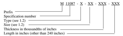
Example of part number M11087I06280228 (i.e., 19 feet long 6.625 O.D. x .280 in. wall pipe with both ends grooved.)
