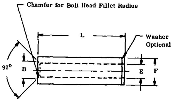
Ends of bushing and bushing plus washer to be flat and parallel within .002. Surface texture of ends: 32 microinches per ANSI B46.1
