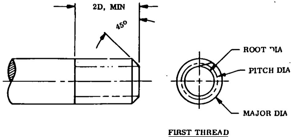
**DETAILS:****MATERIAL: STEEL****HARDNESS: HEAT TREATED TO ROCKWELL C60 to 64.**
