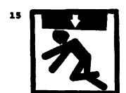
HEAVY PARTS - heavy object on human figure shows that heavy parts present a danger to life or limb.
