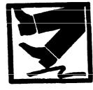
SLICK FLOOR - wavy line on floor with legs prone shows that slick floor presents a danger for falling.
