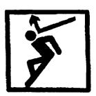
FALLING PARTS - arrow bouncing off human shoulder and head shows that falling parts present a danger to life or limb.
