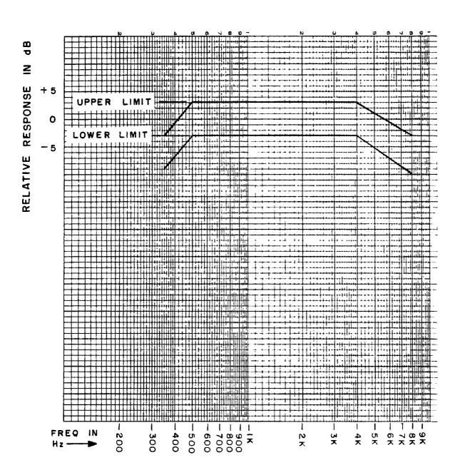
FIGURE 1. Frequency response - limit curves.
