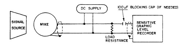
FIGURE 3. Impedance measurement schematic.
