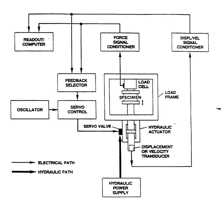
FIGURE 2. Schematic diagram of major components of electrohydraulic closed-loop test machine
