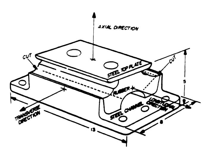
FIGURE 5. Sketch showing axes of type 5B5,000H resilient mount and location of cuts for porosity and delamination test
