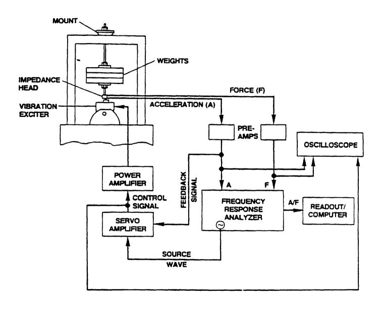
FIGURE 1 Typical system for measurement of resonant frequency by the suspended mass method.
