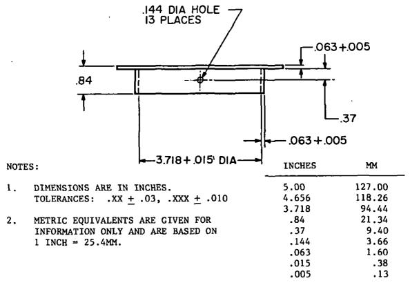
FIGURE 4. Typical mounting flange dimensions and configuration.
