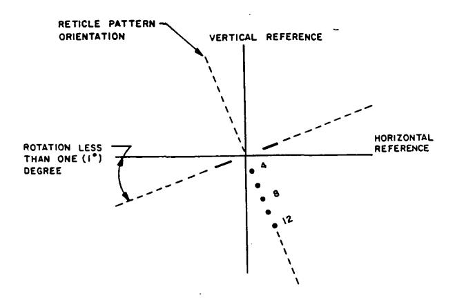
FIG. 4. RETICLE PATTERN ORIENTATION
