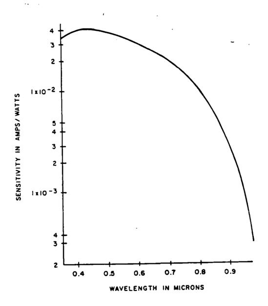
FIG. 1. S-20 EXTENDED RED RESPONSE CURVE
