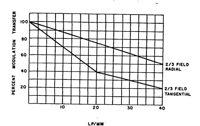
FIG. 3. OBJECTIVE MTF OFF AXIS
